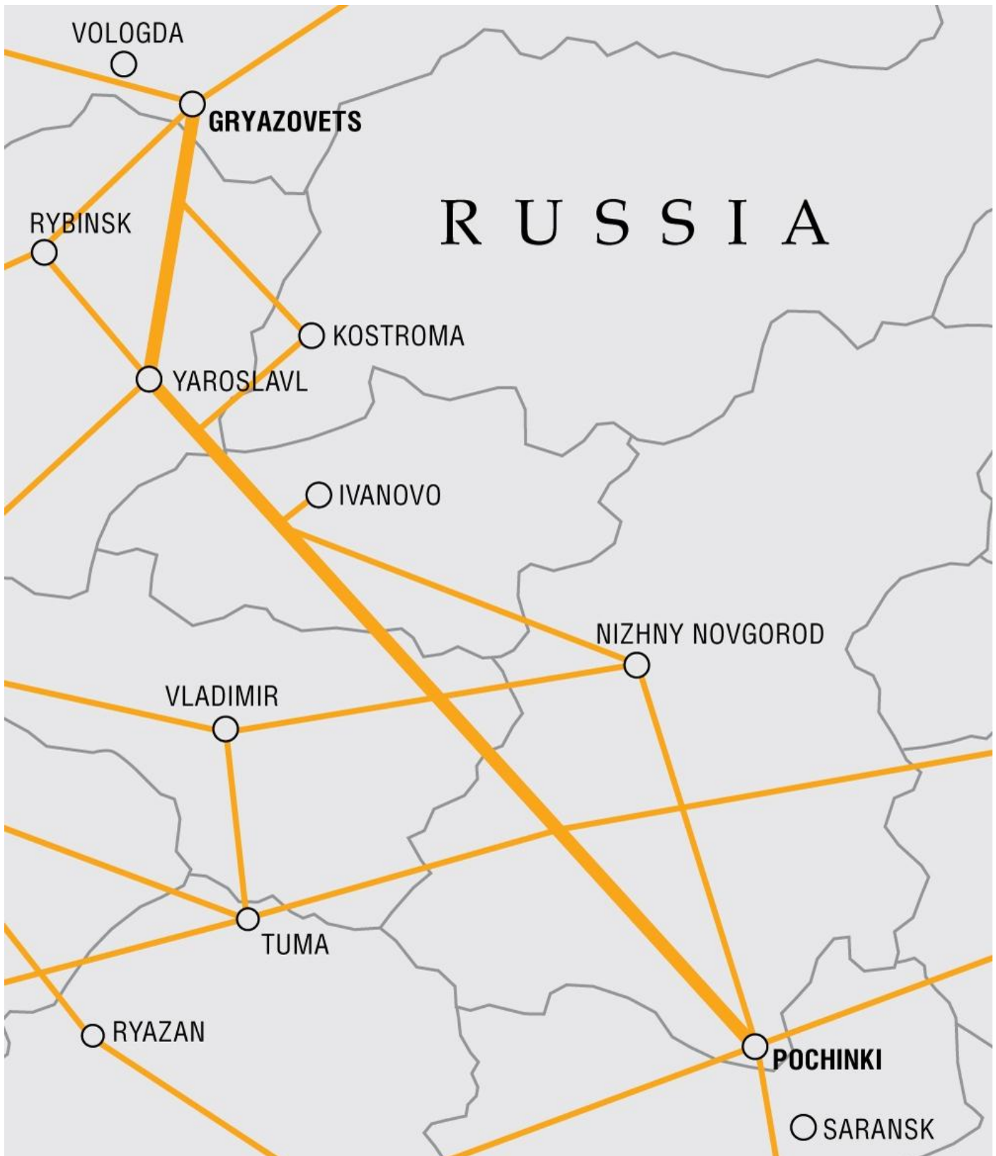
Fig.2. New gas pipeline connecting Gryazovets and Pochinki
